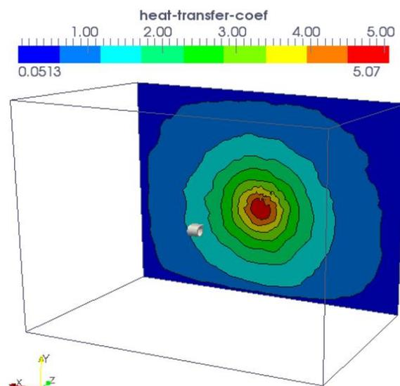
**Figure 2. Convective heat transfer coefficient [W/(m<sup>2</sup>K)] distribution over isothermal surface for TFV 10 S fan for a wall distance of 3500 mm.**
