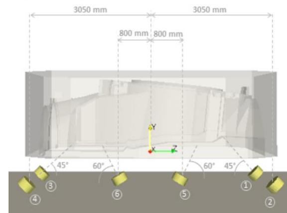
Figure 10. Optimal fan arrangement for main foundation mould.
